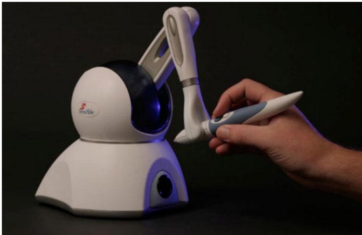
ZScan 700 and Sensable Omni Haptic Arm, use to scan and modify data for digital models
